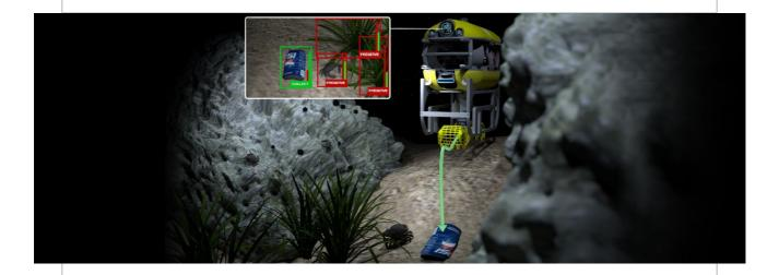
A robotic system intended to clean litter from the seafloor has passed its first real-life tests in waters near Dubrovnik, Croatia. The cleaning system, which works similarly to home robot vacuums, was able to see waste on the bottom of the sea and move towards it. A plastic bottle became the first official litter to be picked up from the seabed. This series of tests is a small step in humanity's goal of cost-effectively cleaning the seafloor, where more than 90% of the sea garbage is found.
